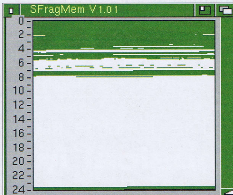
A4000 memory allocation - note the gaps at the start vacated by earlier programs and QuickROM's 512K 'reverse' allocation at the end.
